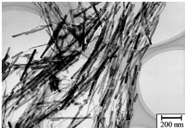
FIGURE 4 TEM image of \alpha -Fe 2 O 3 nanorods liberated from carbon nanotubes by O 2 gasification at 600°C.
